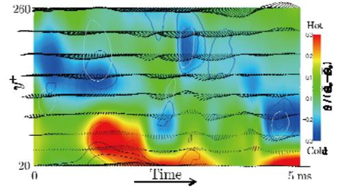
Instantaneous velocity vectors and temperature fluctuations measured by multi-wire probe composed of submicron cold-wires (*IJHFF*, 2008)
