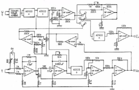
Analog circuit for simultaneous measurement of velocity and temperature fluctuations (*JHT*, 1978)
