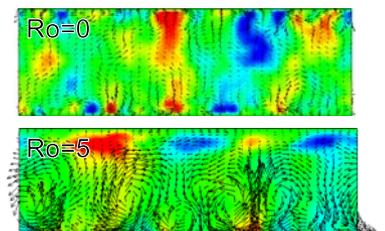
Streamwise averaged velocity vectors and temperature fluctuations in non-rotating/rotating channel flows by DNS of spectral method (*JoT*, 2003)
