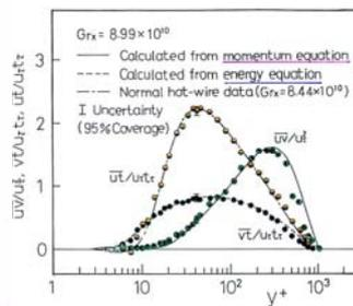
Reynolds shear stress and turbulent heat fluxes in natural convection TBL (*IJHMT*, 1988)
